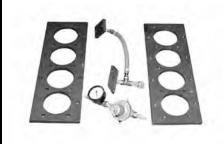
Used to check porosity of cylinder block in rebuilt engines (Engine blocks often become pitted on outer wall of cylinder due to improper cooling system maintenance. If pitting becomes severe and cylinders are bored oversize when the engine is rebuilt, there is a possibility that the cylinder wall can have porosity not noticed by visual inspection alone.)
