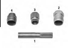
Use the extractor and wrenches to remove and install fuel injection pumps and retaining bushings
