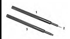
Used for installing piston cooling orifices and plugs
