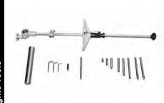
Provides very accurate measurements, which are compared to block specifications, to determine how much of top surface of cylinder block has been machined (when an engine is reconditioned, it is important to know if top deck has been previously machined)
