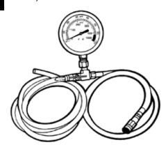
• Used to measure fuel pressure, take a fuel sample and check for aerated fuel.
